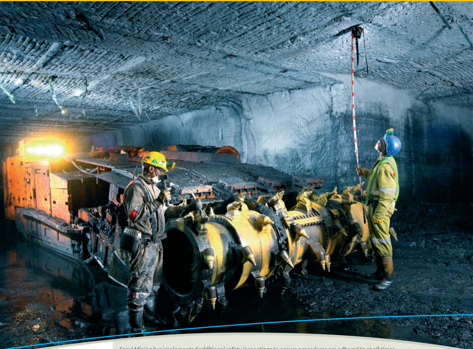
Sasol Mining has implemented additional safety inspections to ensure procedures are adhered to at all times. Edward Mafutwane checks for the presence of flammable gases at Twistdraai Colliery.
